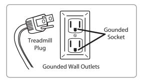
**Danger:** Improper connection of the equipment grounding conductor can result in the risk of electric shock. Check with a qualified electrician or service person if you are in doubt as to whether the product is properly grounded. Do not modify the plug provided with the product. If it will not fit in the outlet, have the proper outlet installed by a qualified electrician.
